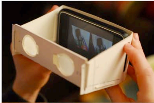
Viewer with device inserted with "side by side" media playback
